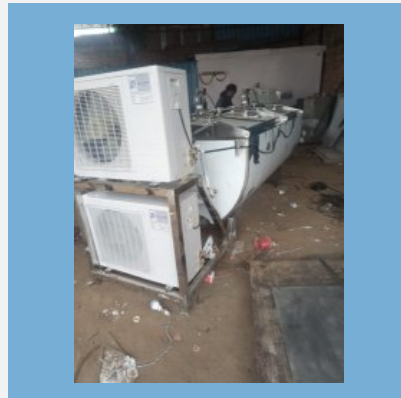
Bulk Milk Cooling Tank Of 2000 Ltr. With Double Compress0r
